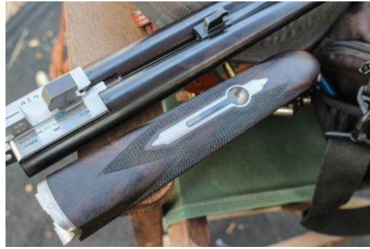
The splinter forend gave a positive grip, with none of the bulk of the larger beavertail forend designs.
